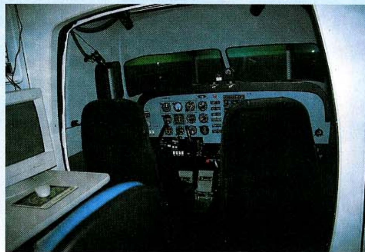
The simulator was "parked" at the end of the Boise, Idaho, runway for these photos. Note the complete Bendix/King Silver Crown package. The single-engine power quadrant exchanges in seconds for a twin quadrant and the cover plates, as seen on the EGT, are removed.
